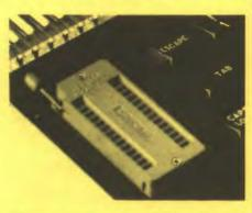
Allows you to change your ROMs quickly efficiently, without opening the lid. The ZERO INSERTION FORCE (ZIF) socket is located into the ROM Cartridge's position.
